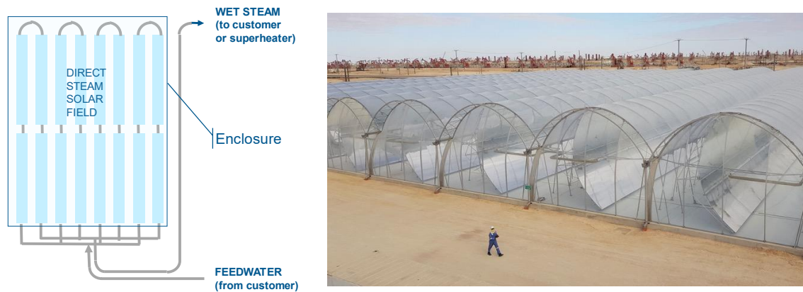
Figure 5. Enclosed parabolic trough collectors for direct steam generation (left: schematic, right: photo).
